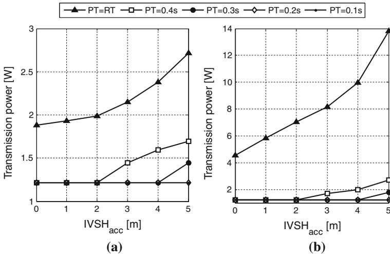
**Fig. 8** Required transmission power to exchange at least one CAM before CD and before CD + ED with probability  $p = 0.9999$  considering realistic positioning for  $IVS_m = 10$  m,  $RT = 0.75$  s,  $v = 70$  km/h and 100 Bytes payload. **a**  $N = 2$ . **b**  $N = 5$
