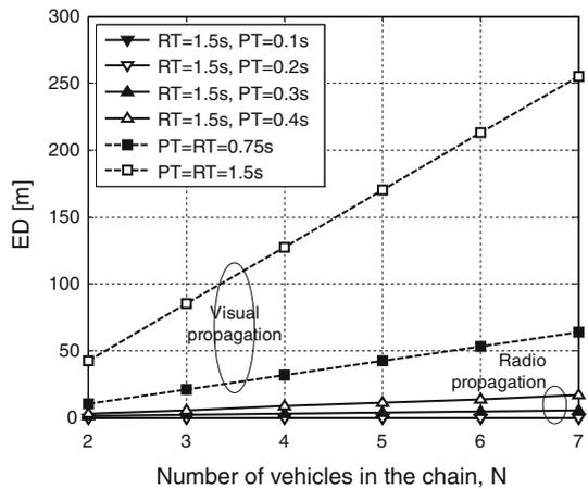
On the other hand, the *ED* distance required to avoid chain collisions can be quite significant at high speeds and at short *IVS* distances, especially for high driver’s reaction times.
