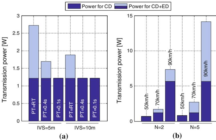
**Fig. 7** Required transmission power to exchange at least one CAM before CD and before CD + ED with probability  $p = 0.9999$  considering 100 Bytes payload. **a**  $v = 70 \text{ km/h}$ ,  $N = 2$  vehicles and  $RT = 0.75 \text{ s}$ . **b**  $IVS = 5 \text{ m}$ ,  $RT = 0.75 \text{ s}$  and  $PT = 0.4 \text{ s}$
